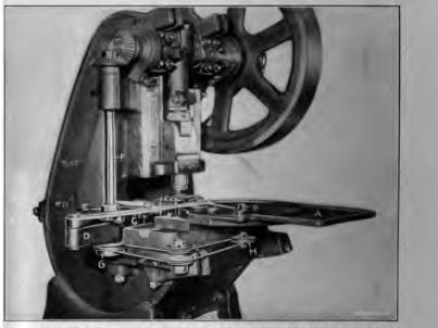
Fig. 11. Press Equipped with Combination Friction-dial and Push Feed
